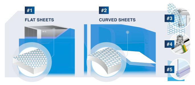
1 Flat panels offer better electro-static dissipation 2 Curved panels offer less efficient electro-static dissipation 3 Potential equipotential bonding by hinge 4 Ground connection Al-profile (ESD) 5 Grounding by panel element
